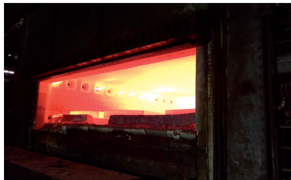
Fig. 9 Shuttle kiln No. 3 in service at 1280 °C
