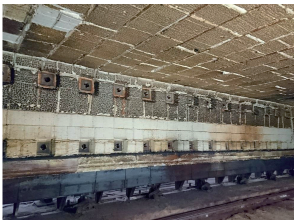
Fig. 2 Typical appearance of lining after several years of operation, here shuttle kiln No. 1
